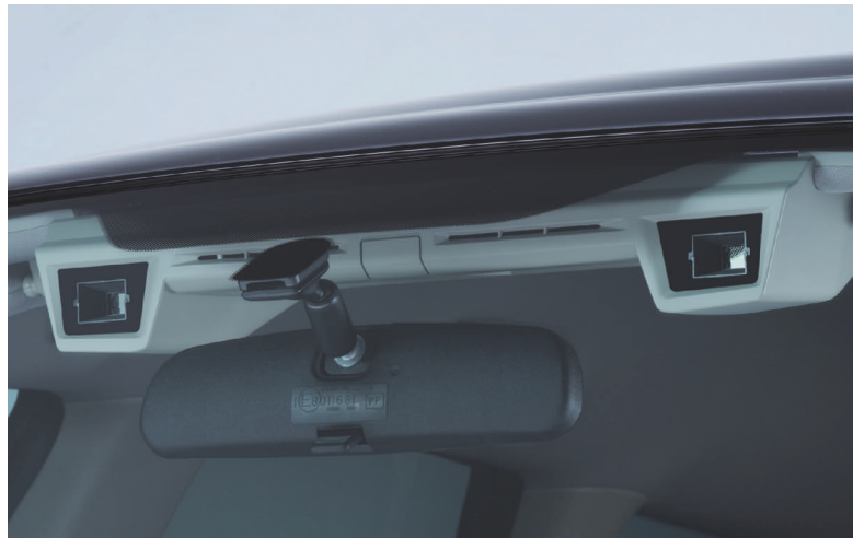
FIGURE 1 The Eyesight stereo camera sits above the rearview mirror. The space between the right and the left cameras is 350 mm (courtesy FHI).
